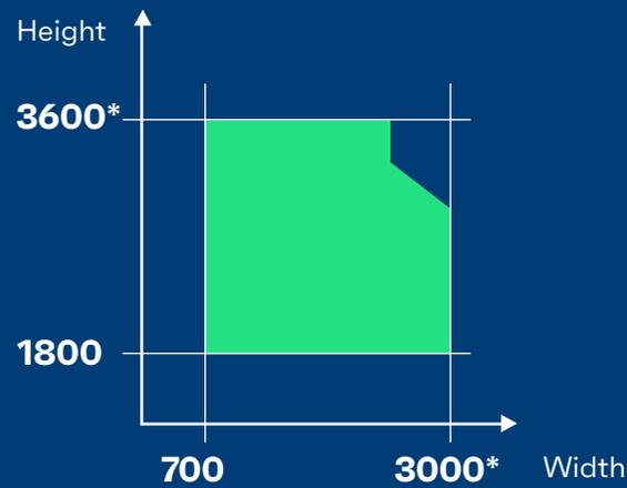
\*Max dimensions depend on multiple parameters including wind load requirements and glass type choice.
